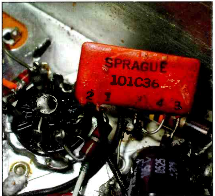
Photo F. The square module with the numerous leads is the Sprague Couplate. This contains the resistors and capacitors that provide the RC coupling between the audio stages.
