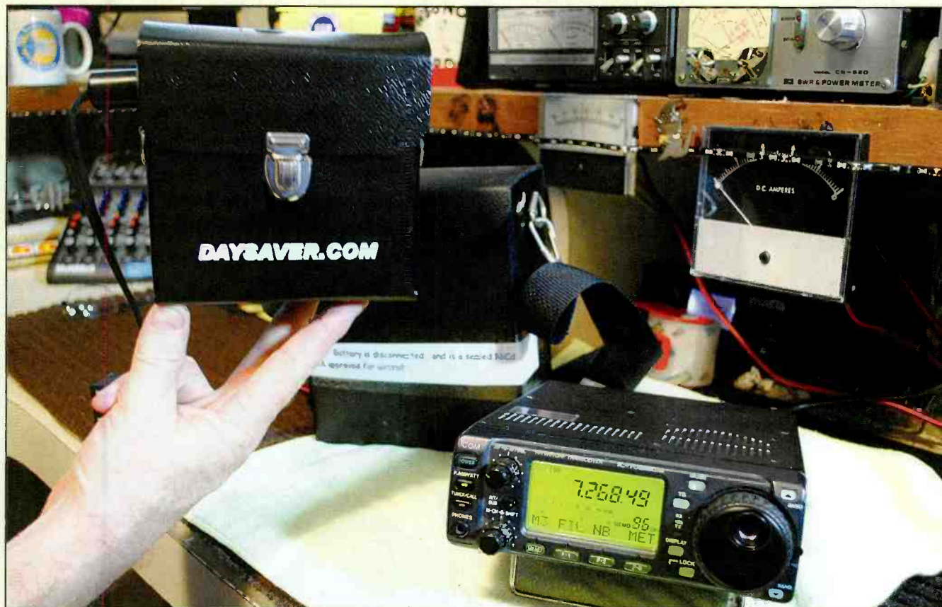
Photo J. The new DaySaver lightweight Lithium Iron Phosphate battery, seen in the foreground, is half the size of the lead-acid battery to the rear — and one-fifth the weight. Yet, the two batteries have the same capacity. (Courtesy of WPC6NOA)
