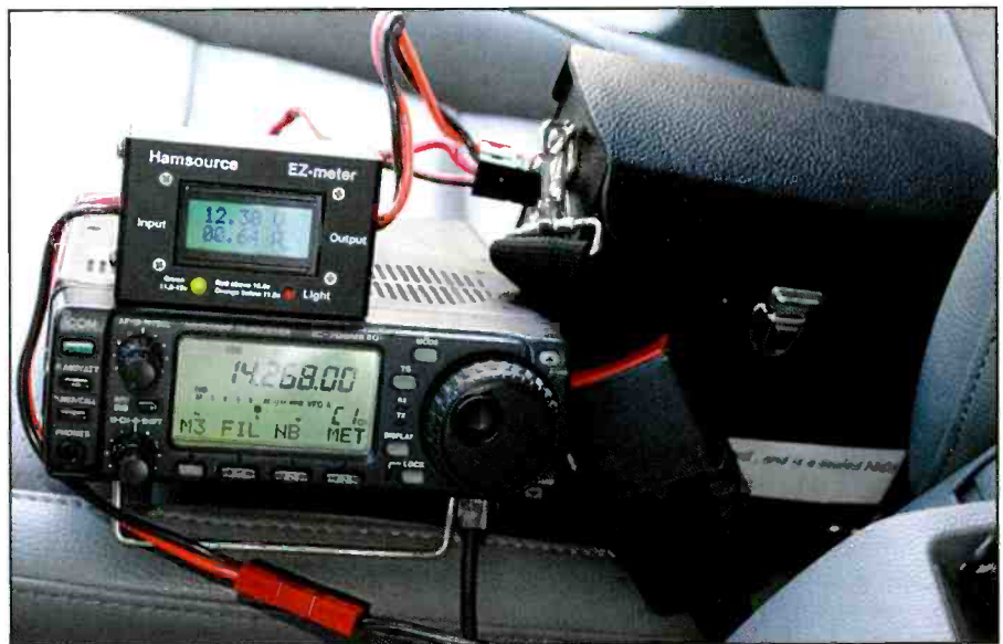
Photo C. HamSource has a digital combination volt meter and ampere meter that when placed in series with the Anderson connector output along with the HamSource power supply/voltage isolator, is perfect for maintaining the 10.5-amp-hour sealed battery.
