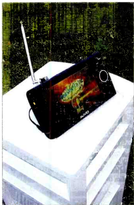
Photo 1. In testing, the whip received four Baltimore stations — one poorly and three well. Meanwhile, the KPC3FL Turnstile-Bowtie-Gain DTV Antenna, “up a little higher — about four feet — was able to improve on that and received three new stations poor or a bit better and 11 stations well,” he said.
