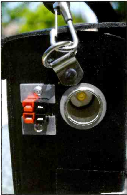
Photo B. The 10.5-amp-hour sealed lead-acid battery from Daysaver is used as a “buffer battery” between the rental car’s power socket and WB6NOA’s radio gear. It features twin-Anderson connectors, built-in overload circuit breaker, and the round accessory power socket. It is housed in a handy carrying case with strap.
