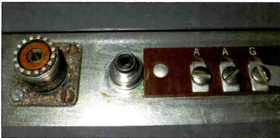
Photo C. An RCA jack was added to the rear apron on this receiver, allowing access to the recovered audio from the detector stage. This can be used with an external amplifier to provide bass and treble control. I try to find an existing hole that will accept the RCA jack to avoid drilling the chassis.
