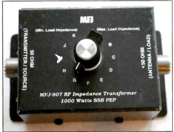
Photo H. This MFJ Enterprises impedance matching bridge is used at WB6NOA/M on 40 and 20 meters to achieve a low SWR with no other tuner needed.
