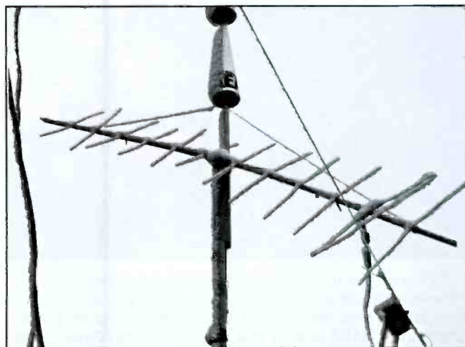
Photo F. This snow-covered 12-element Yagi at KPCØUFO is used to track space debris and orbiting objects detected by the USAF Space Fence.
