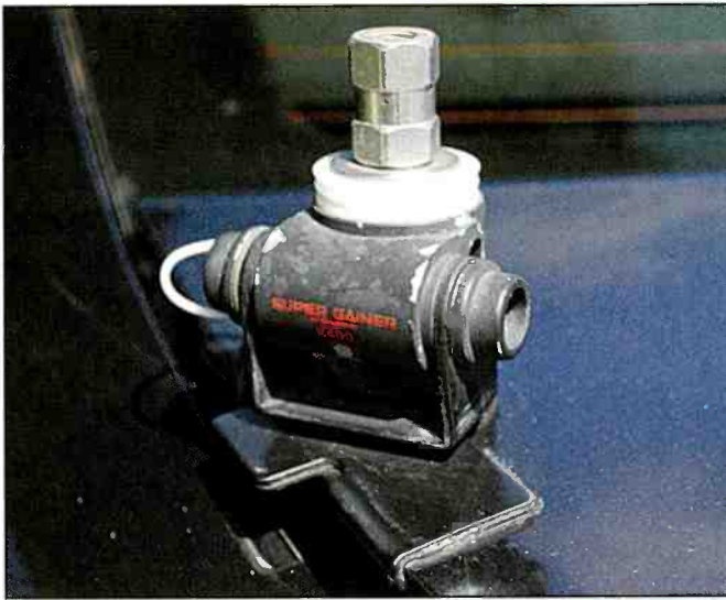
Photo G. The Diamond K-400 antenna mount can slip over a rental car's trunk lid with ease.
