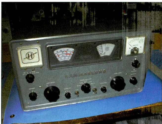
Photo A. Here is “Farmer Rik’s” HQ-100 receiver. The Auto Response circuitry is being removed to improve the radio’s audio response. (Photography courtesy of K1ZJH)
